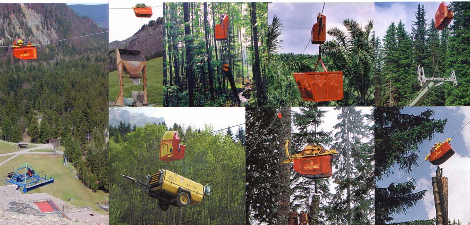
Carrying cable supports for longer distances.
